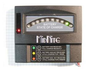
On the above display the green LED indicates the battery has 90% of full charge. The red LED behind the tinted cover indicates the battery has not been fully charged for at least 2 weeks.
